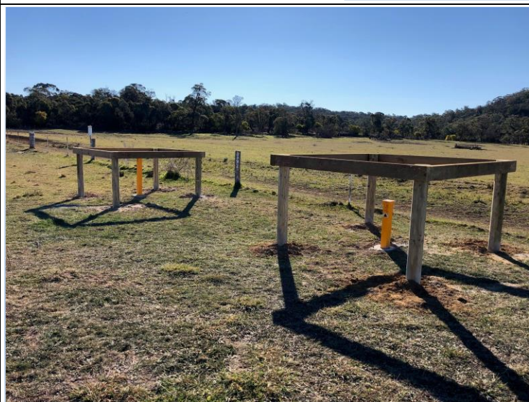
Plate 3: STK20S and STK20D Piezometers Completed Source: Austral Bricks
