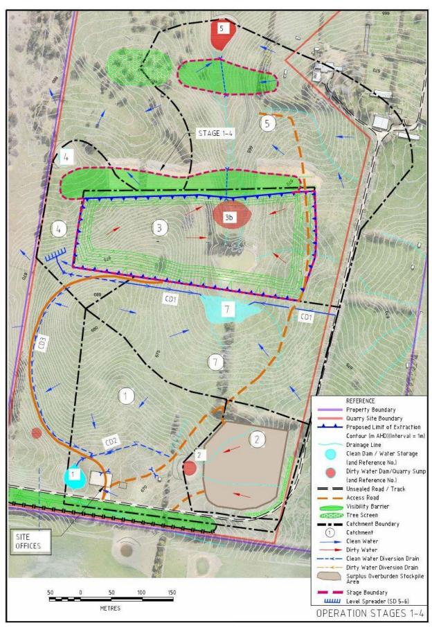
Figure 7 Water Management: Stages 1-4 Operation
