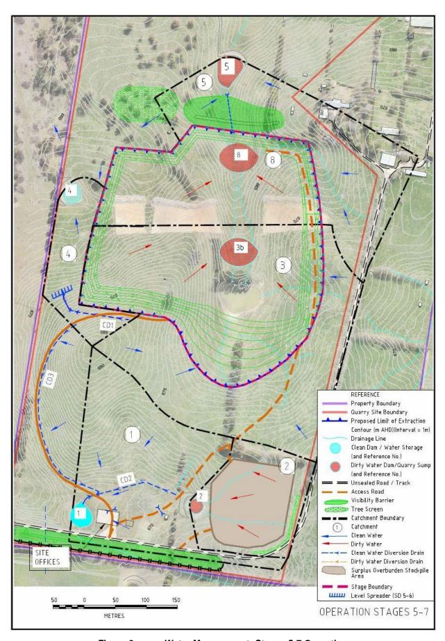
Figure 9 Water Management: Stages 5-7 Operation
