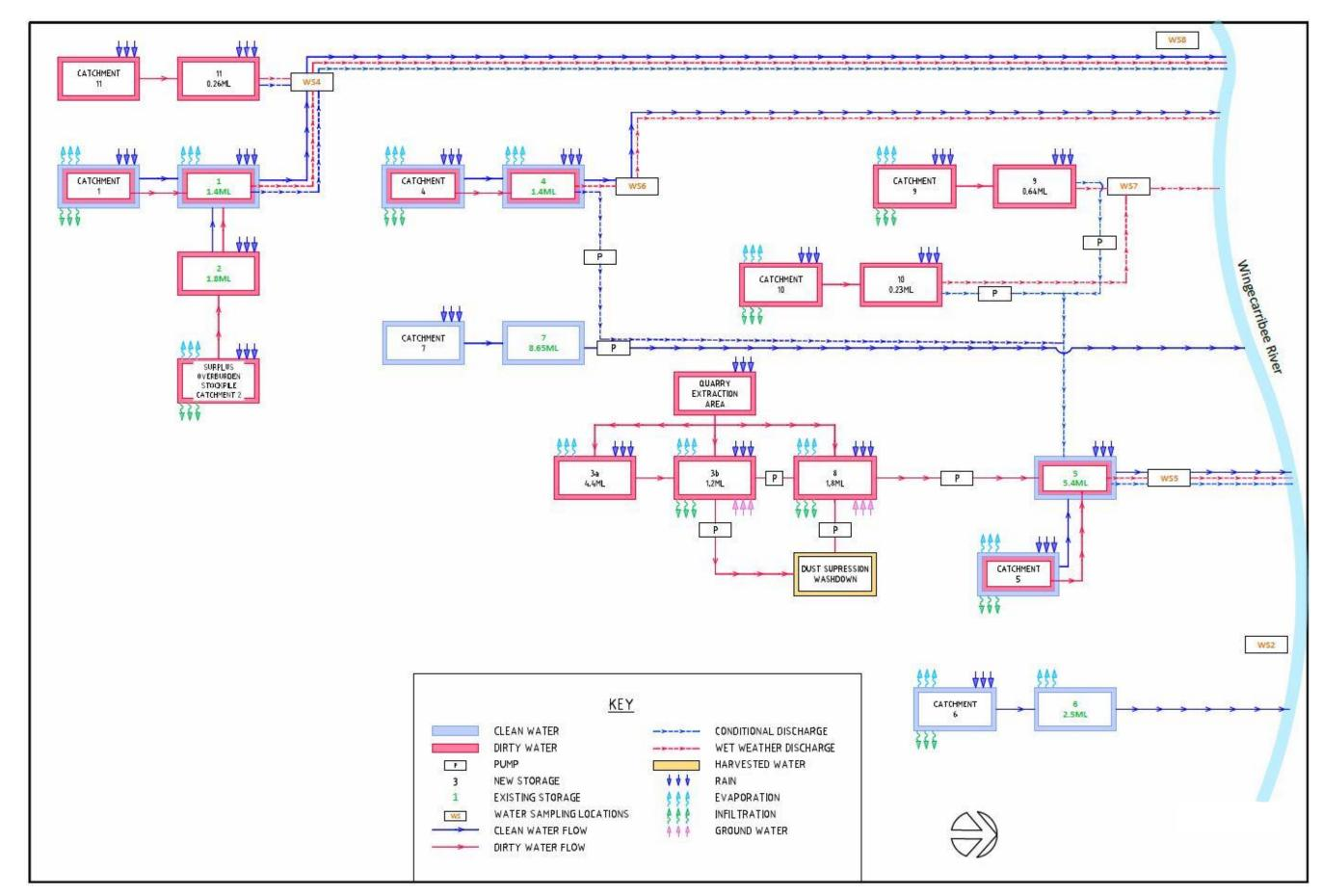
Figure 5 Site Water Balance Flow Chart
